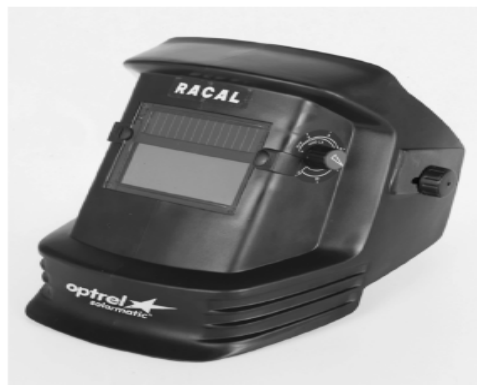
Fig. 1 Helmet with electronically controlled filter, powered by solar cells above the viewing aperture, with knob adjustment of the effective shade number.
