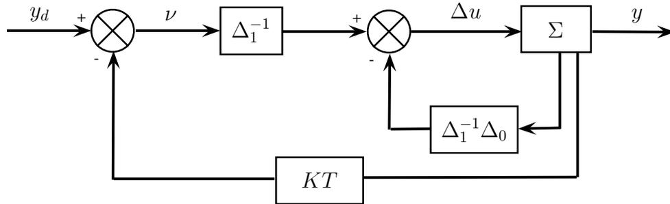
**Figure2.** Stabilization of the decoupled MIMO system
