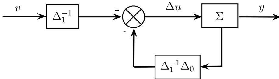
**Figure1.** Decoupled MIMO system
