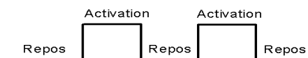
Fig.6. Classic paradigm of activation for the survey in BOLD. An alternation of phases of activation and rest (or reference) is used. [2][11]5. TREATMENT OF THE DATA
