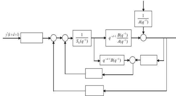
Fig. 1. Structure of the stabilizing controller parametrization.
