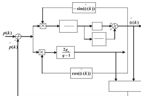
Fig. 5. Structure of the Magnitude Phase Locked Loop MPLL.
