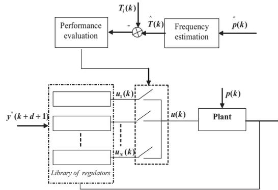
Fig. 6. Structure of the multiple disturbance rejection.
