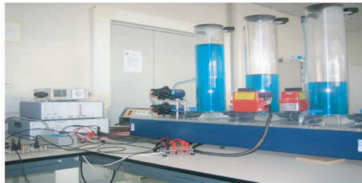
Fig. 2. Laboratory experiment : Thre tank system
