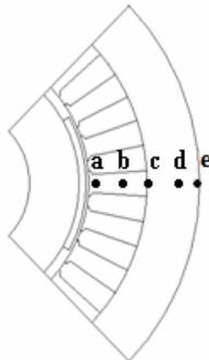
Figure 2: Points for which the flux density have been computed
