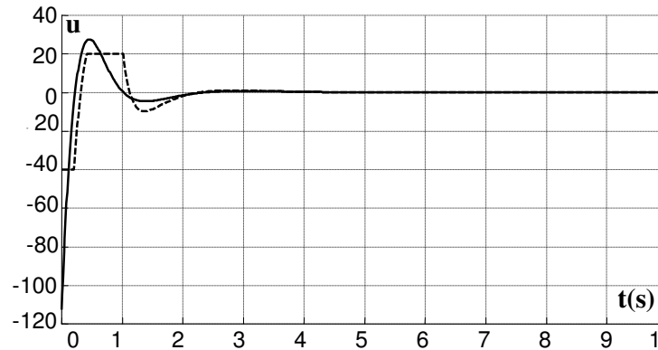
Fig. 3. This figure show the evolution of control input (-.- : system with saturation, - : system without saturation constraint). We can notice that the control is saturated and always inferior to its maximal values. Also it shows a typical stable sliding mode convergence.
